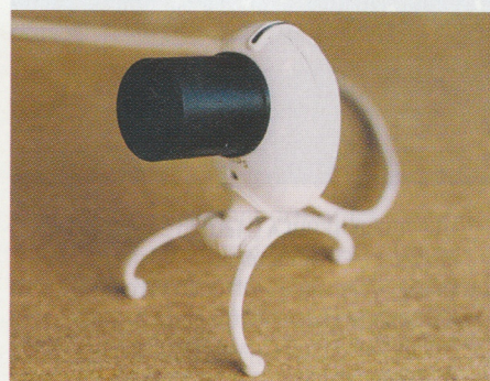
THE PHILIPS ToUcam PRO 740K has the ability to take quality astroimages even in its unmodified form. Add the Mogg telescope adapter [right] to connect the webcam to a telescope. KEITH WILEY
